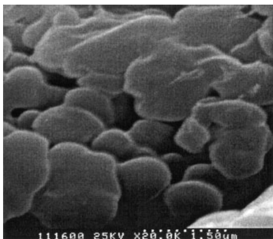
Figure 2 SEM micrograph of PVC primary particles.
