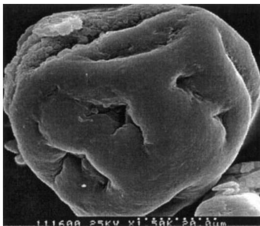
Figure 1 SEM micrograph of a PVC particle.
